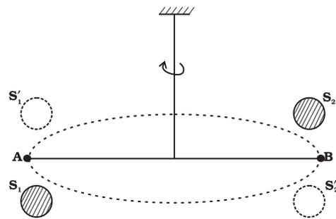
**Fig. 7.6** Schematic drawing of Cavendish's experiment.  $S_1$  and  $S_2$  are large spheres which are kept on either side (shown shades) of the masses at  $A$  and  $B$ . When the big spheres are taken to the other side of the masses (shown by dotted circles), the bar  $AB$  rotates a little since the torque reverses direction. The angle of rotation can be measured experimentally.
